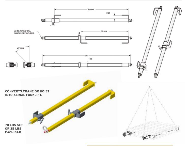
\*\* FOR A LEVEL LIFT, THE CENTER LIFTING BAIL MUST BE OVER THE LOADS CENTER OF GRAVITY
