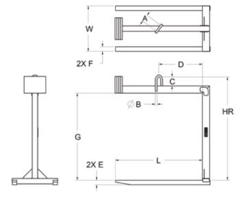
\*\* FOR A LEVEL LIFT, THE CENTER LIFTING BAIL MUST BE OVER THE LOADS CENTER OF GRAVITY
